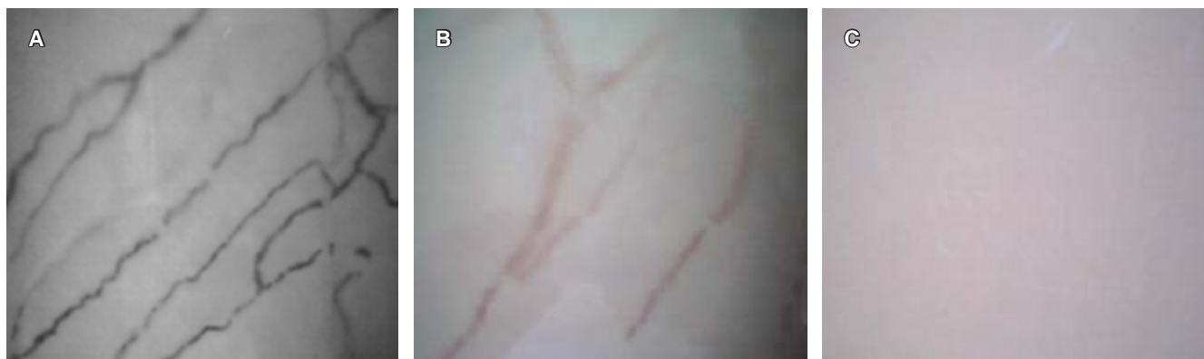
Figure 2: A) (24 hours) shows a rectangular segment of bovine pericardium treated only with 0.5% glutaraldehyde. B) 7 days. C) 15 days with the treatment based on 0.5% glycine for 24 hours. Residual glutaraldehyde is practically zero.
