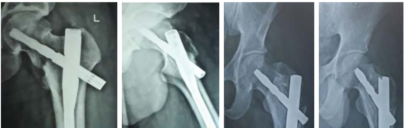
Figure 8: Radiographic series of left hip showing locking mechanism failure of a long helical screw.
