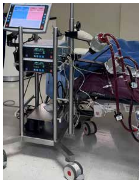
Figure 3: Biventricular mechanical extracorporeal cardiac support with a dual CentriMag axial flow system (Levitronix GmbH, CH-8048 Zurich, Switzerland).
